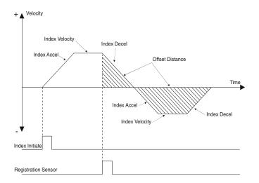
*Figure 47: Registration to Sensor Profile (Offset < 0)*
